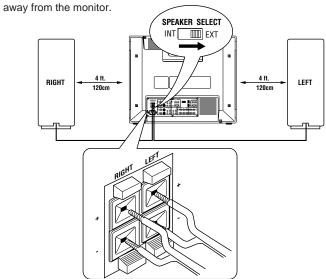
**CAUTION:** Unplug the monitor and all connected components before connecting external speakers. Use only speakers with 8-ohm impedance and a power output rating of 5 watts or more.
